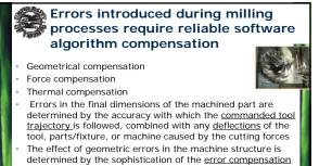
algorithms The cutting tools' trajectories are subject to <u>performance of</u> <u>the axis drives</u> and the <u>quality of the control algorithms</u>
